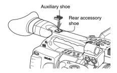
Place the auxiliary shoe on the rear accessory shoe and secure it with the four screws.
